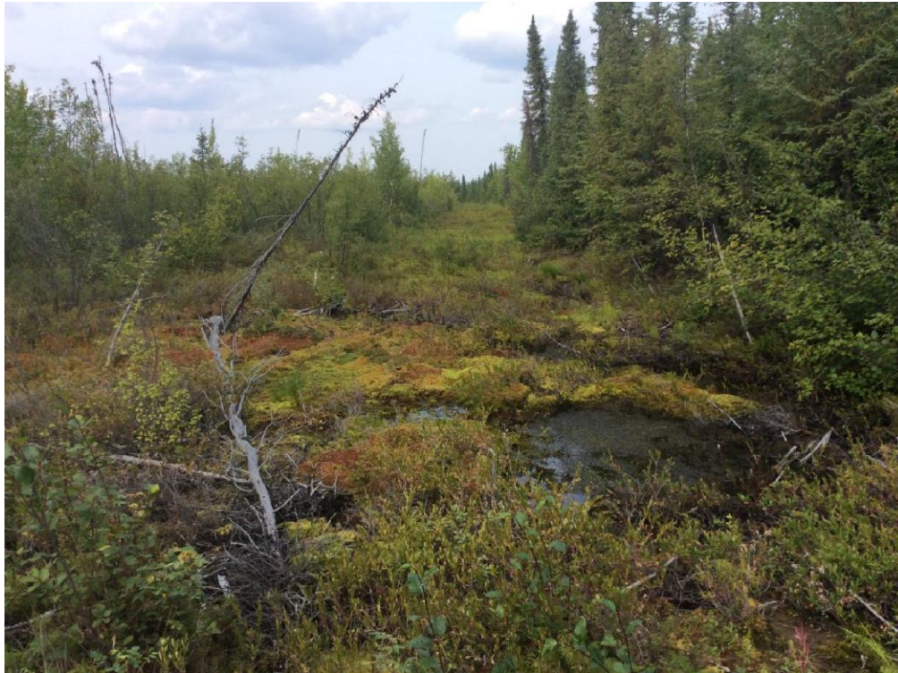
Attachment Photo A-21. Ground survey plot SL243, a burnt winter road with melt pockets present, indicating permafrost degradation.
